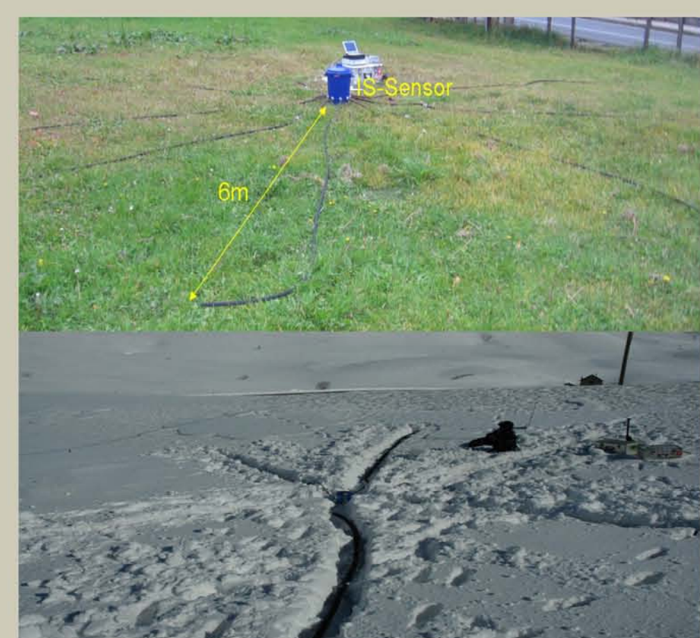
Figure 1: The array setup, 8 porous garden hoses encased in a perforated pipe in a star configuration. Top: Summer setup Bottom: Winter setup.
