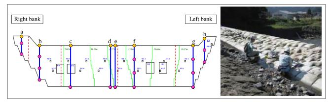
Fig. 11 Elastic wave exploration
