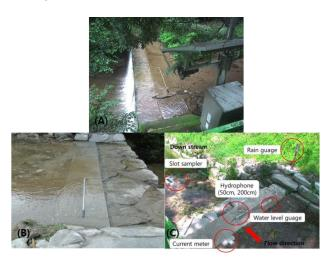
**Fig. 1** Site photos of the bedload monitoring sites (A: Control site, B: Landslide site, C: Forest fire site)
