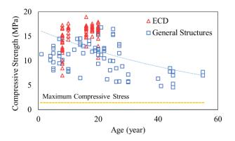
**Fig. 9** The result of comparison between compressive strength regarding strength reduction factor (0.55) and maximum compressive stress multiplied by safety factor (2.0). In addition to same symbol to **Fig. 7**, yellow dash line means maximum compressive stress.
