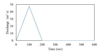
Fig. 4 Simplified hydrograph for initial input data of Kanako 2D
