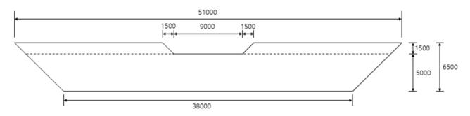
Fig. 1 Dimension of modeled erosion control dam from front-view (unit: millimeter).
