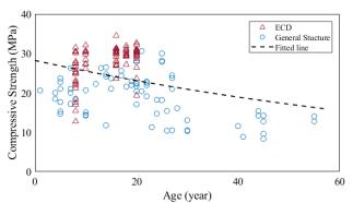
Fig. 7 Aging degradation model derived from results of previous studies [*Koo et al.*, 1994; *Kim et al.*, 2000; *Song et al.*, 2010; *Park et al.*, 2013]. Red triangle means data from ECD measurements [*Park et al.*, 2013]; blue square means general structure researches [*Koo et al.*, 1994; *Kim et al.*, 2000; *Song et al.*, 2010].
