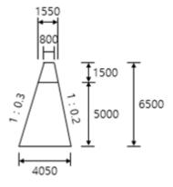
Fig. 2 Dimension of modeled erosion control dam from side -view (unit: millimeter).
