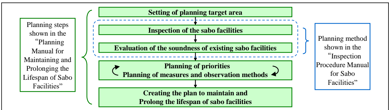
Fig. 8 Contents of the “Planning Manual for Maintaining and Prolonging the Lifespan of Sabo Facilities” and the “Inspection Procedure Manual for Sabo Facilities”
