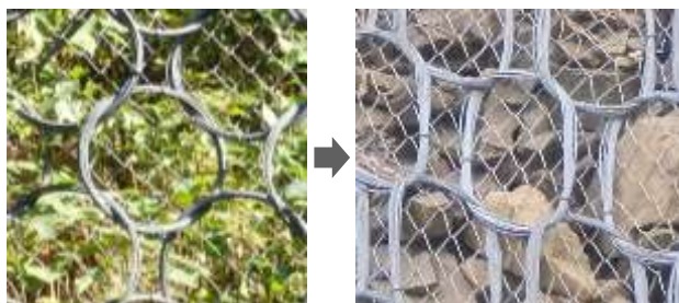
Fig. 3 Deformation of ring net - (left) unloaded, (right) loaded
