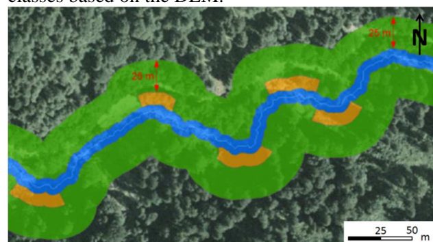
Fig. 4 Identification of process-relevant areas: Windthrow-affected areas with a distance of one tree-length from the channel are depicted in green. The areas related to erosion of forest covered riverbanks are shown in blue. Bank erosion related-areas are plotted in orange. In this example, no landslide reaches the channel
