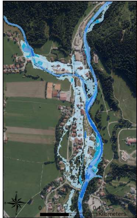
Fig. 14 Simulation result for the scenario considering a log jam at the bridge at Entfelderstrasse. The Entfelderstrasse bridge's position is marked with a green dot. The bridge at Alpenstrasse is marked with a red dot
