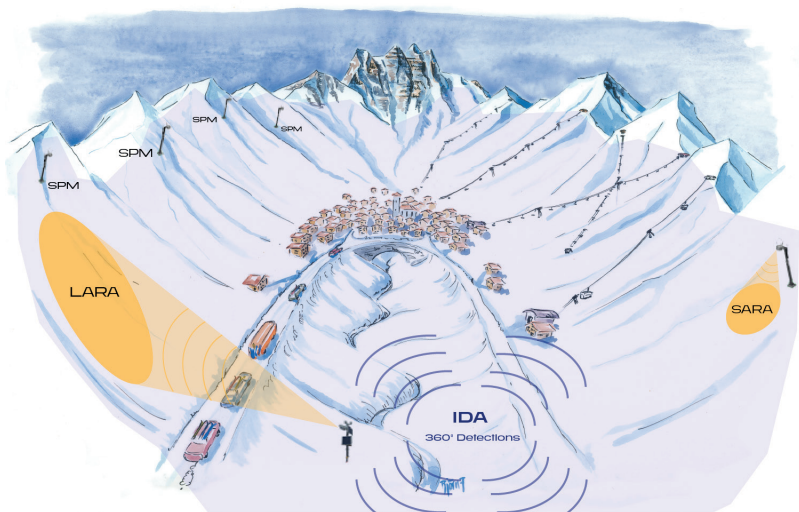
Figure 1: Schematic overview of operational radar (LARA, SARA) and infrasound (IDA) detection systems.
