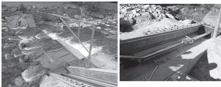
Figure 1: (left) the measuring station: the array of geophones is installed on half width on the downstream end of the check dam and (right) a detail of the turbidimeter installation system
