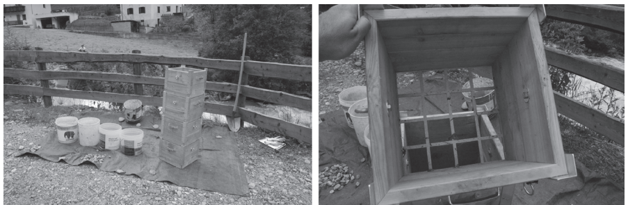
Figure 3: (left) sieves used to separate coarse pebbles (64mm, 45mm, 32mm and 22mm) from medium-fine pebbles (<22mm), (right) a detail of the 64mm sieve
