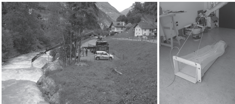
Figure 2: bedload sampling using a crane mounted trap (left), the sediment trap (right)
