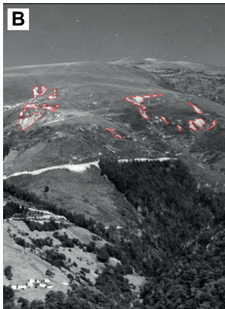
Figure 2: Example of mapping on an oblique terrestrial photograph. A) Georeferentiation and orthorectification of a terrestrial oblique photograph with the WSL-Monoplotting-tool: example of the Alpe Rompiago study area in 1923. B) Shallow landslides in the Alpe Rompiago study area in September 1941. C) The landslides shown in B) reported by the WSL-Monoplotting-tool on a 2012 orthophoto. Photographs ©CVC; orthophoto ©swisstopo.
