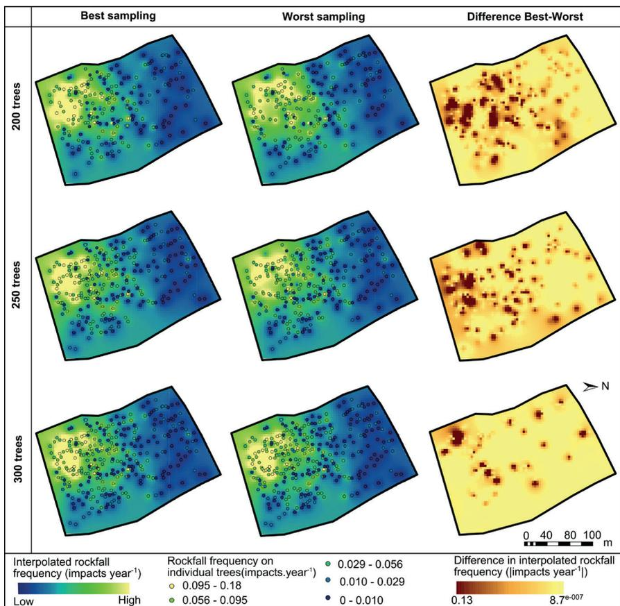
Figure 3.2: Best (lowest RMSE, left panel) and worst (highest RMSE, central panel) rockfall frequency maps interpolated for each of the 100 subsamples of 200 to 300 randomly extracted trees. Maps on the right panel represent the differences in absolute value between the best and the worst frequency maps computed for each subsample.
