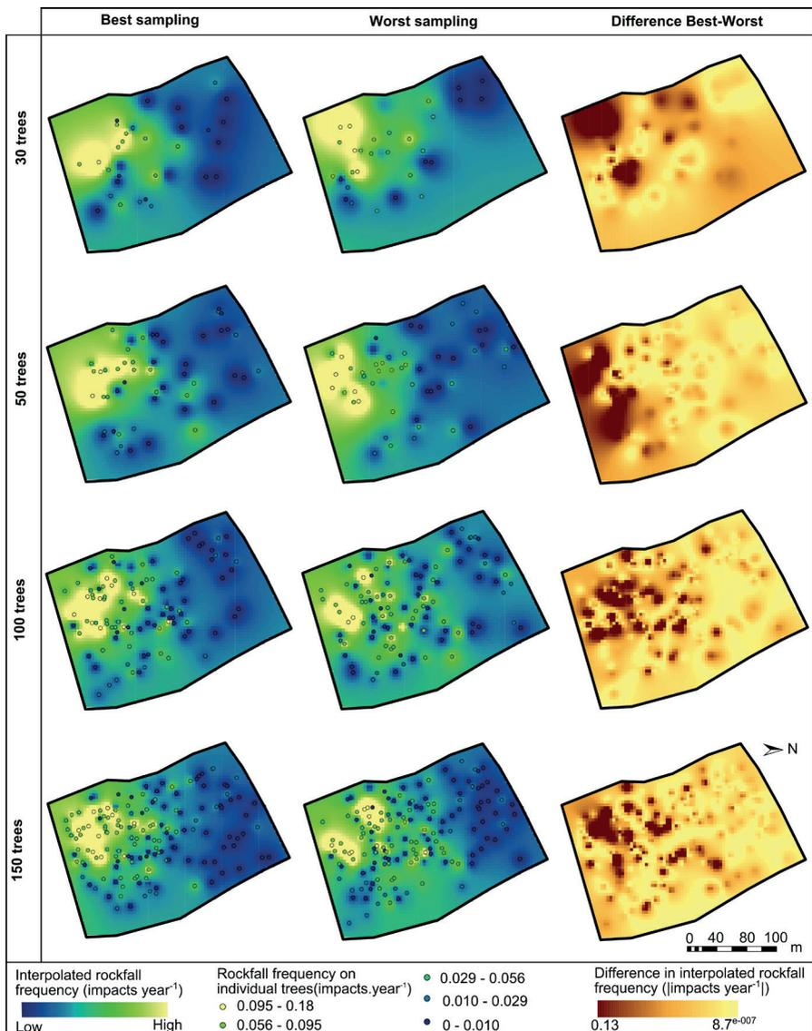
Figure 3.1: Best (lowest RMSE, left panel) and worst (highest RMSE, central panel) rockfall frequency maps interpolated for each of the 100 subsamples of 30 to 150 randomly extracted trees. Maps on the right panel represent the differences in absolute value between the best and the worst frequency maps computed for each subsample.
