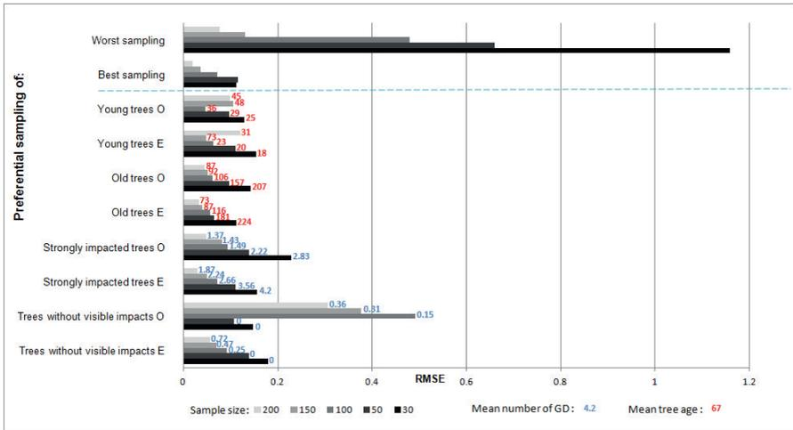
Figure 8: Root Mean Square Error (RMSE) measuring the deviation of frequency maps generated with different subsets from the reference frequency map. RMSE is given for various sample sizes and worst random extractions as well as for different arbitrary selections. Preferential sampling in areas with heterogeneous rockfall activity is presented by 'E' and in homogeneous by 'O'.
