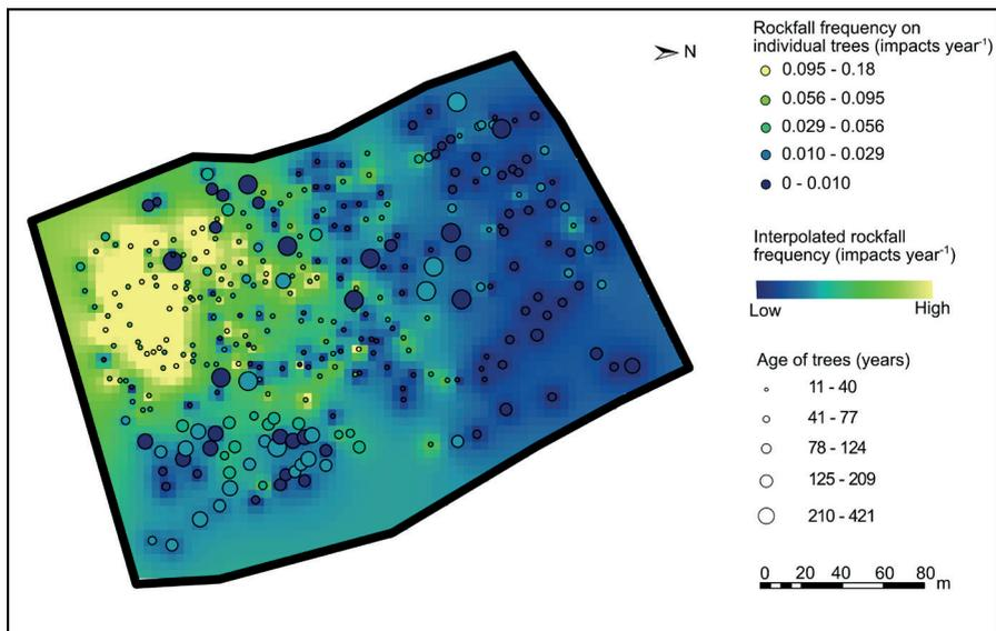
Figure 2: Reference frequency map (Refmap) of rockfall derived from the 314 sampled trees. The interpolation was performed using inverse distance weighted method.
