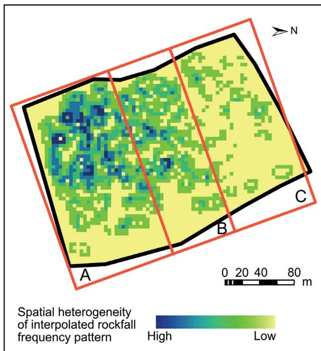
Figure 7: Heterogeneity map computed from Refmap using the ArcGis spatial statistics tool “slope” (ESRI, 1998) that calculates the maximum rate of change in value from one cell to its neighbors. Rectangle delineates the three compartments (A) homogeneous, (B) intermediate and (C) heterogeneous used respectively weighted 0.1, 0.3 and 0.6 in the stratified sampling strategy.
