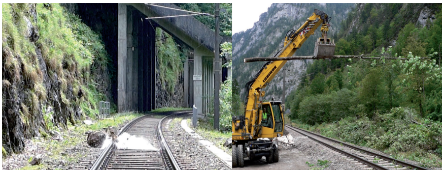
Figure 3: Left: Rocks thrown down on railway tracks. Right: Simulation of tree-fall using an excavator.
