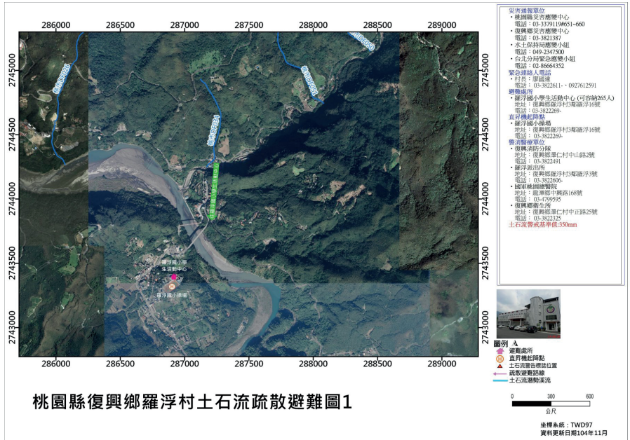
Figure 1: Evacuation route map of Holiu village near potential debris flow torrent (blue line, No. TaoyuanDF034). Shelters, moving directions, helicopter landing area, and other information of hospital, police station, fire department, emergency operation center, and emergency contact person are all indicated in the map.
