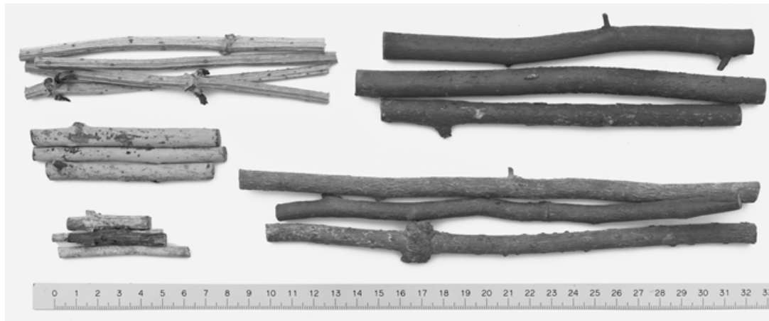
Fig. 4 Photograph of the driftwood classes, in model scale 1:40, measuring tape in (cm)
