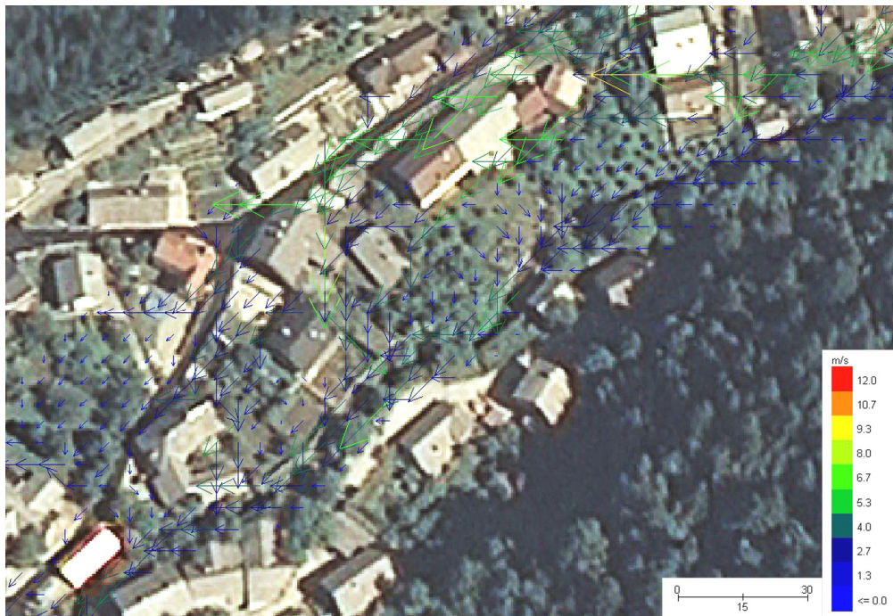
Fig. 3 Maximum velocities (vectors) using blocked (“dry”) cells for representing structures (the upper part of the fan).
