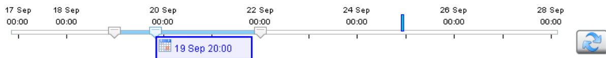
Fig. 1 Time slider: inner (with calendar date) slider is used to set the map, bulletin and image time; both outer sliders are used to set the time interval for diagrams, tables and warnings (Cockpit); vertical line represents current time; the box with time field and calendar icon shows selected time and can also be used for manipulation; on the right refresh button.
