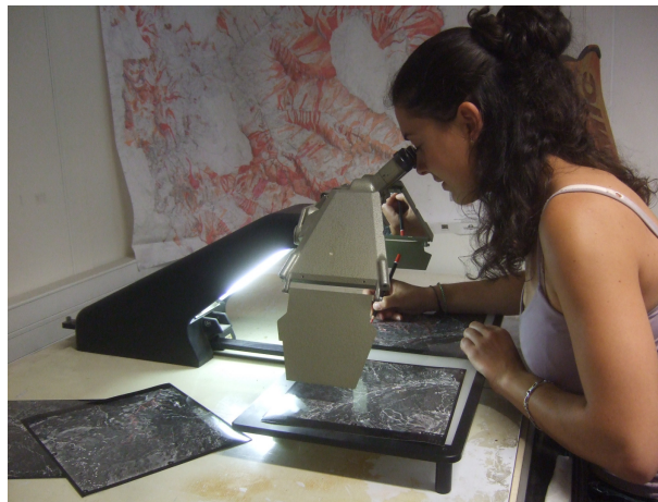
Fig. 3 Photo-interpretation with a stereoscope
