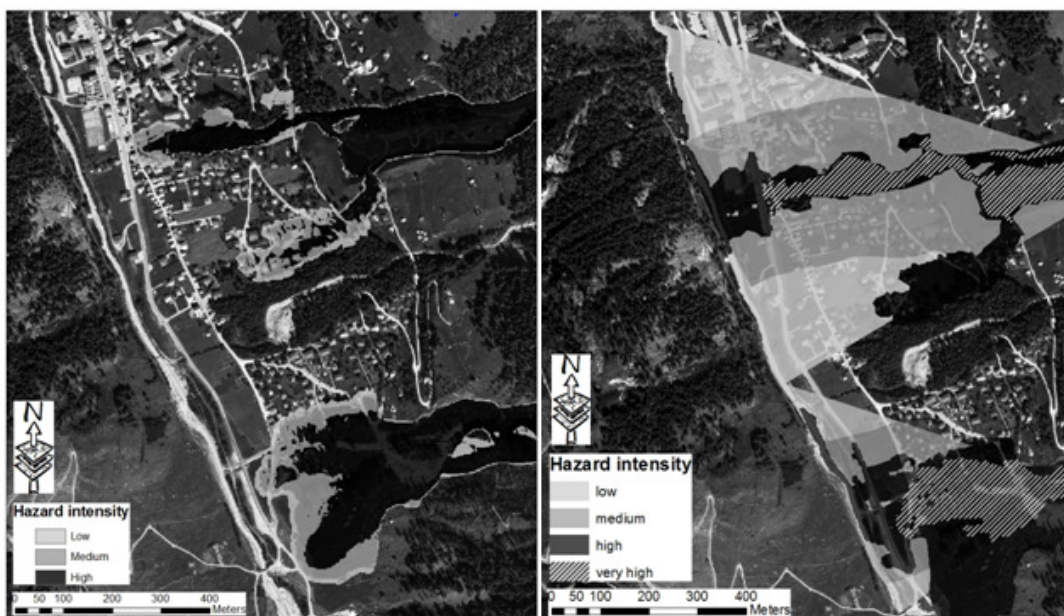
Fig. 3 Comparison between traditional (left) and this study (right) debris flow hazard maps.
