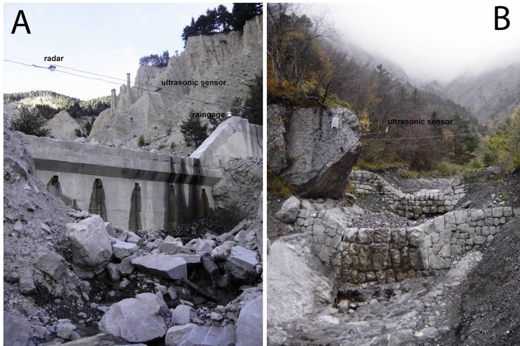
Fig. 2 Examples of two debris-flow monitoring stations deployed in 2010 at the Réal (Réal_S1; Fig. A) and Manival torrents (Manival_S1; Fig. B)
