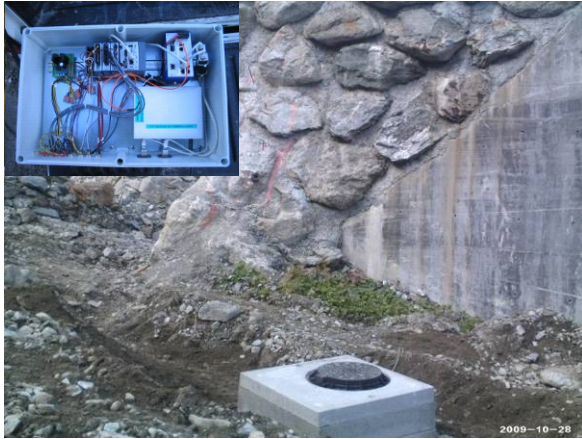
Fig. 8 Data logger and chamber at the foot of the breaking mounds
