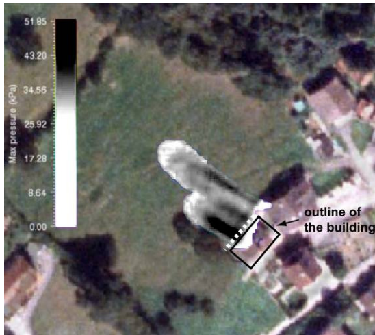
Fig. 2 Debris flow simulation (Alpnachstad / extended Voellmy)
