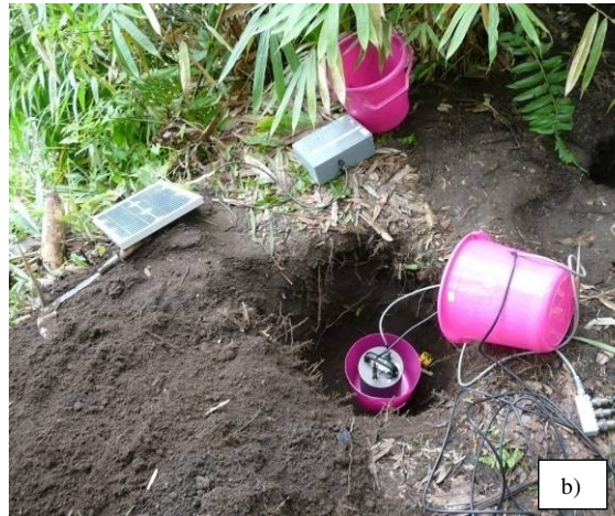
Fig. 4 a) Pore pressure sensor (from Prosensor) and its housing in the bedrock. b) AFM geophone (from Massey University) and a 3 component broad-band seismometer (from Guralp). c) Load cell sensor (from ScotTech-Solinst).
