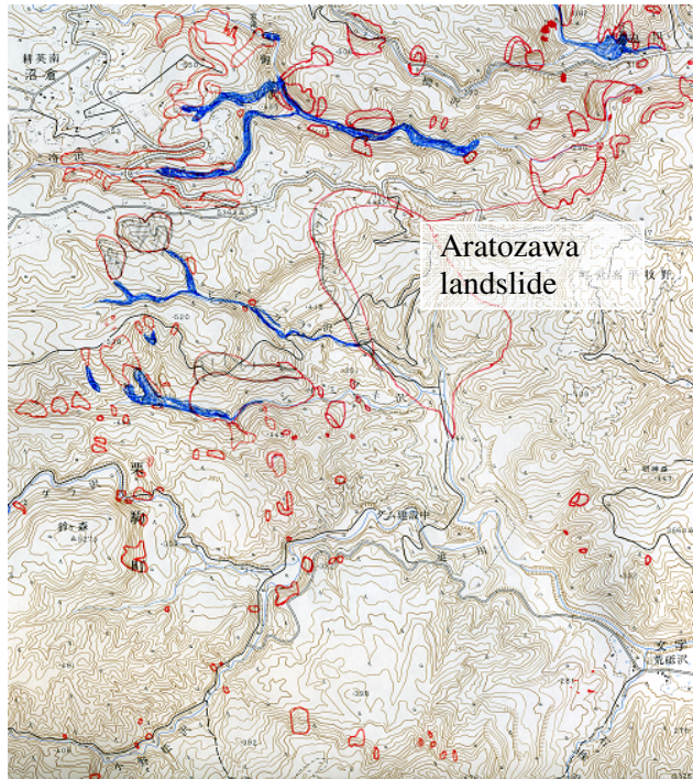
Fig.5 Distribution map of the landslides and slope failures caused by the earthquake (Yagi et al., 2008)
