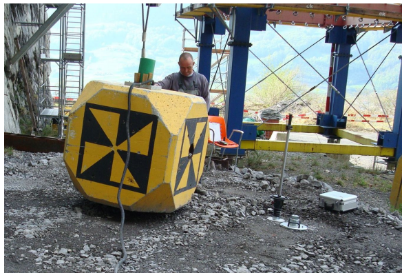
Fig. 1 4'000 kg test block before falling testation
