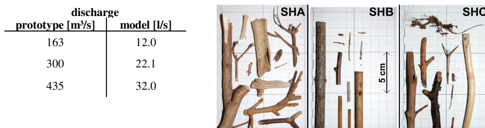
Fig. 3 Physical scale model – left: steady-state conditions; right: driftwood mixtures SHA, SHB, SHC
