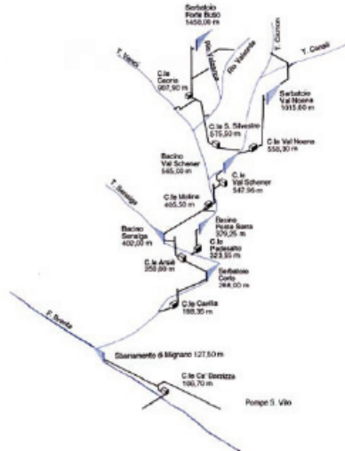
Fig.1: The catchment basin of the Brenta river with dams for hydropower production.
