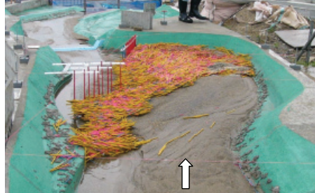
Photo 6. Woody debris trapped using the revised plan.
