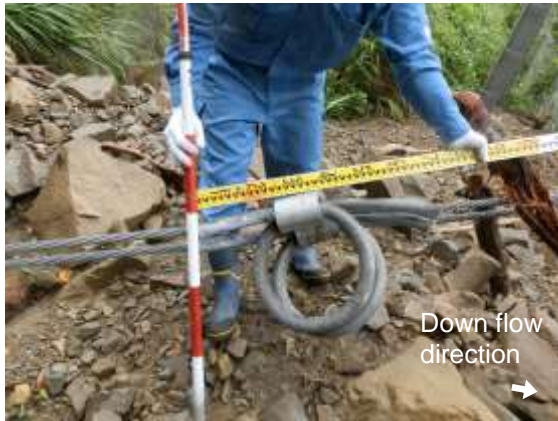
Fig. 17 Measuring the reading of the brake ring travel
