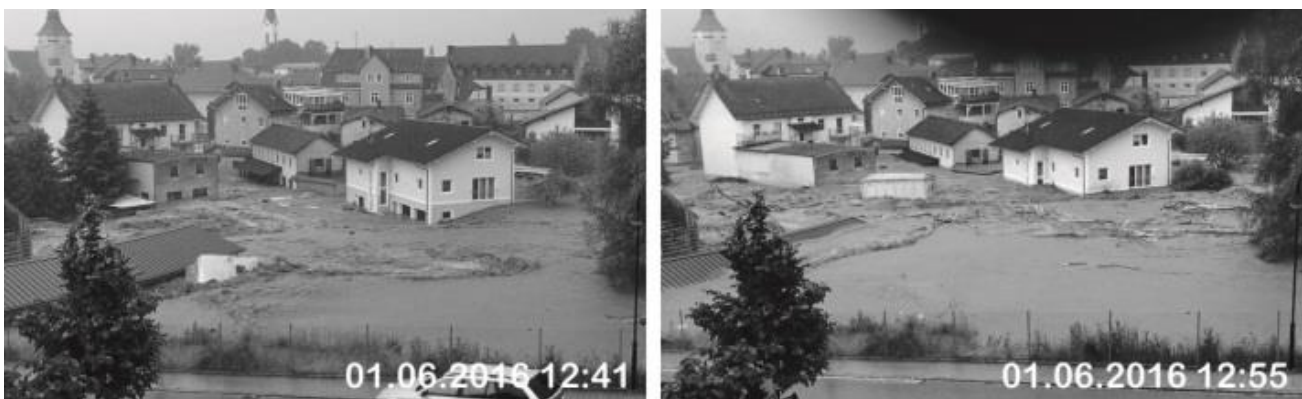
Fig. 6 Discharge at the upper end of the channel through the town about 120 meters upstream of the gauging station. Natural runoff (left) just before the arrival of the breaching surge (right) (Source: Köck)
