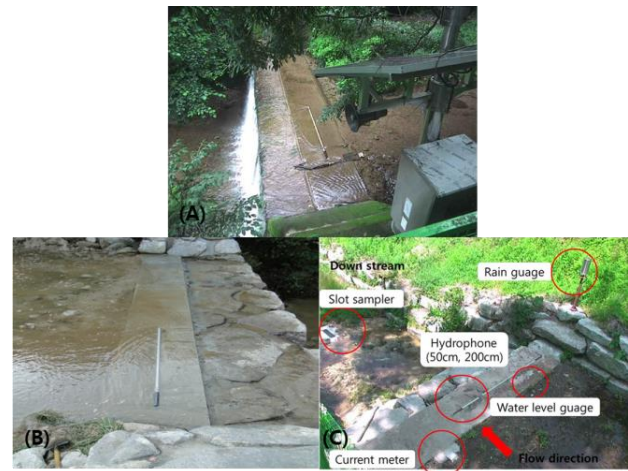
Fig. 1 Site photos of the bedload monitoring sites (A: Control site, B: Landslide site, C: Forest fire site)
