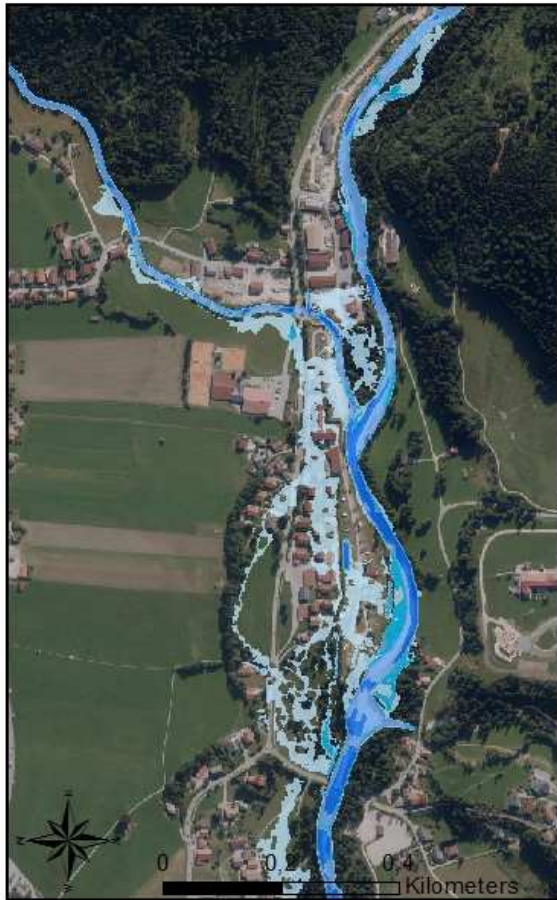
Fig. 13 Simulation result for the default scenario without any log jams or sediment accumulations. The Entfelderstrasse bridge's position is marked with a green dot. The bridge at Alpenstrasse is marked with a red dot
