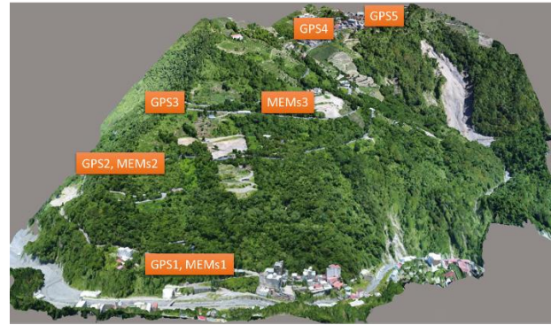
Fig. 9 Locations of dual frequency GPS and MEMs
