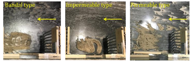
Fig.8 Shapes of sediment deposition corresponding each type of spur dikes
