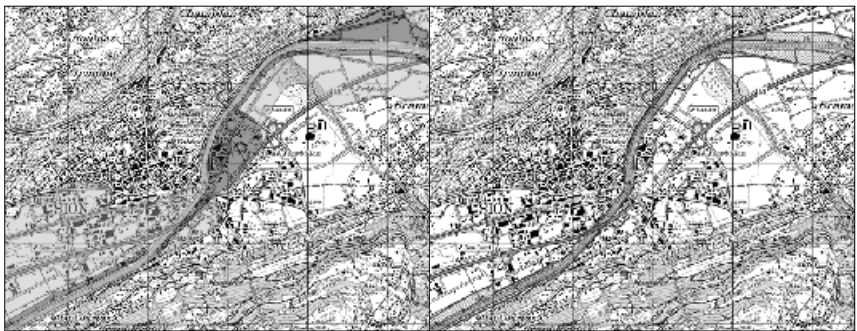
Fig. 1: Sectoral Plan Rhone River showing on the left the hazard index map (dark grey = high hazard intensity, grey = middle to low hazard intensity) and on the right the River Rhone Zone
