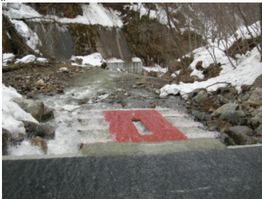
Fig.2: The hydrophone and pit sediment sampler at Ashiarai-dani. The pipe hydrophone was installed 20 cm upstream of the pit.
