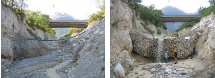
Fig 3: Full scale field test site for ring-net barriers at the Illgraben, Switzerland: Barrier empty (left) and filled (right). On 18.05.2006, 15.000 m 3 debris material flowed through and over the barrier. A volume of 1.000 m 3 was retained, while the rest overflowed the barrier without damaging it.
