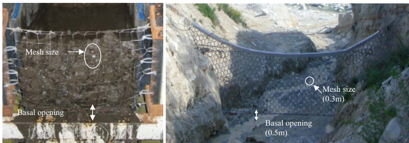
Fig 5: Mesh size and basal opening in the laboratory (left) and in full scale (right).
