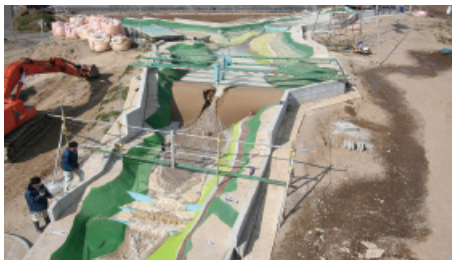
Photo 10. Physical panorama of the model (scale 1/60).
